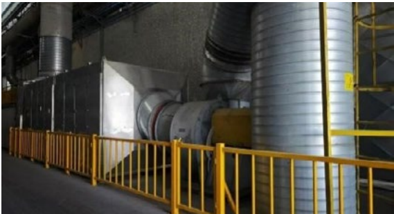
「幹式過濾 + 二級活性炭吸附」VOC 治理設備 "Dry Filtration + Secondary Activated Carbon Adsorption" VOC Treatment System
